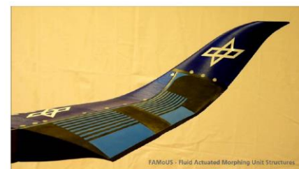
Figure 3: Fluid Actuated Morphing Unit Structure
